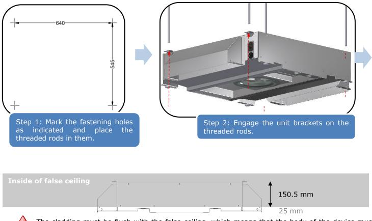
The cladding must be flush with the false ceiling, which means that the body of the device must protrude out of it over at least 25 mm.
