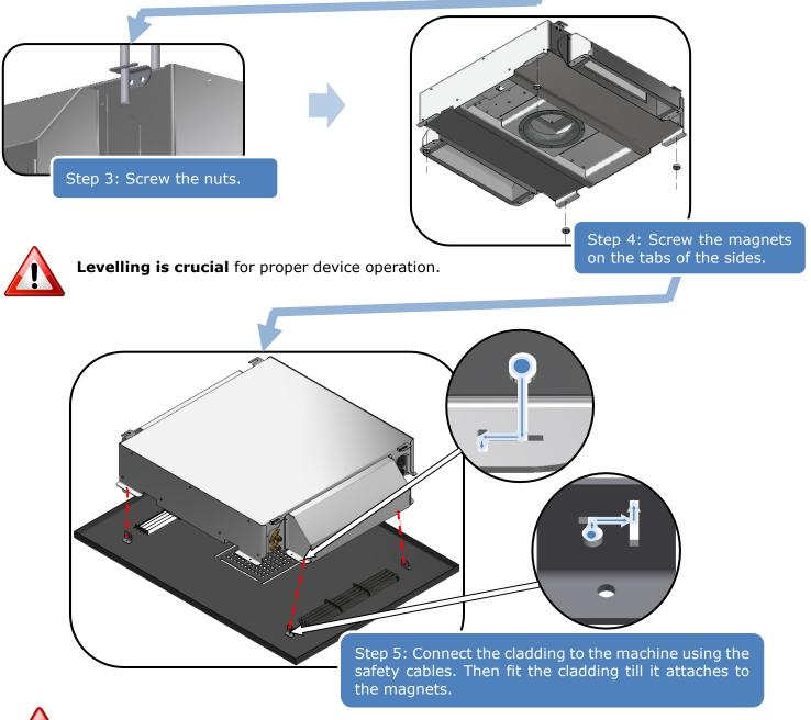
Important: The machine cladding is heavy and must be handled with care <u>even when</u> <u>it is held by the cables</u>!
